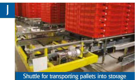
Shuttle for transporting pallets into storage
