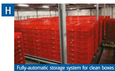
Fully-automatic storage system for clean boxes
